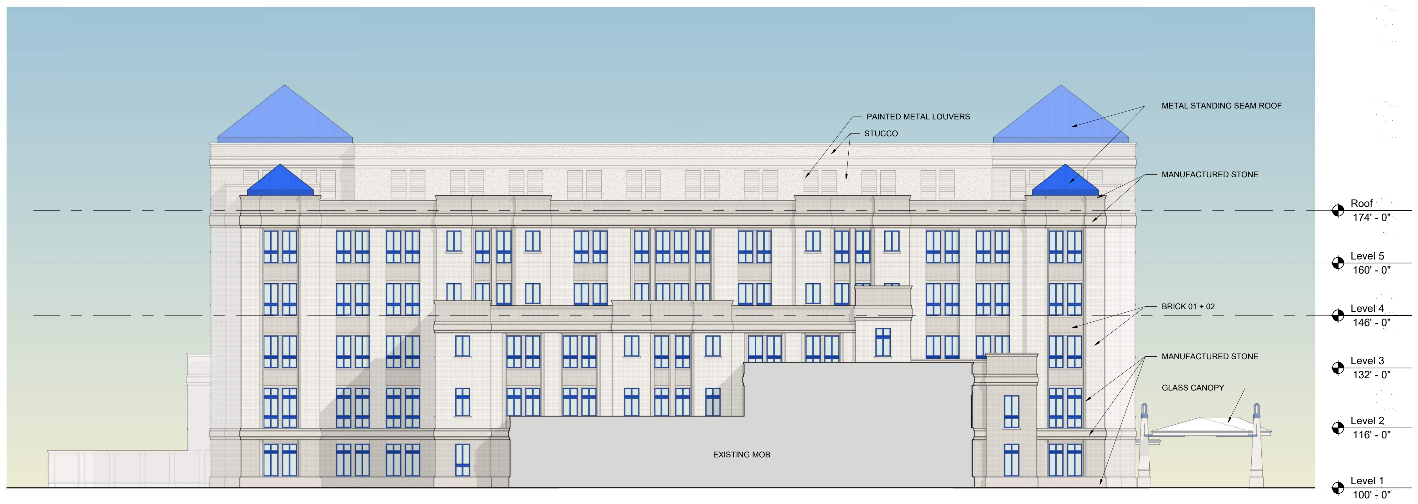
02 WEST ELEVATION - CCMC PROSPER HOSPITAL 1/16" = 1'-0"
